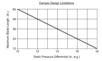
This damper's design at a length of  $60^\circ$  has a maximum allowable blade deflection of L / 360 for the static pressure indicated on the chart. At reduced blade lengths, higher static pressure limits can be attained without sacrificing damper operating performance characteristics.
