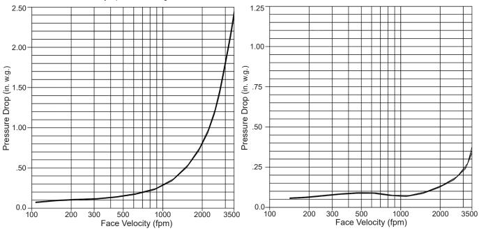
Typical performance for Model PRI9 backdraft damper size tested 42"W x 42"H furnished with counterweight to assist opening.
