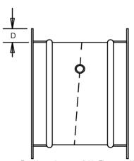
Equal leg angles are available. They are welded to frames at intermittent spacing and caulked between welds. Flange Height "D" varies with damoer diameter.
