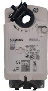
**Description** The OpenAir direct coupled, fast-acting, two-position, spring return electronic actuators are available as 24 Vac/dc, 120 Vac, and 230 Vac models. They are intended for use on UL-listed smoke control dampers and combination fire/smoke rated dampers.
